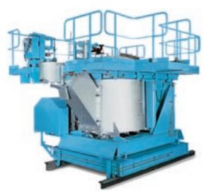
Heated Pressure Pouring Systems are typically used for high production shops where minimal alloy changes are made. They are suitable for gray, malleable and ductile iron and copper-based nonferrous metals. Advantages include:
