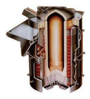
Inductotherm coreless Mini-Heel furnaces maintain a continuous supply of metal ready to pour twenty-four hours a day, seven days a week. They offer:
