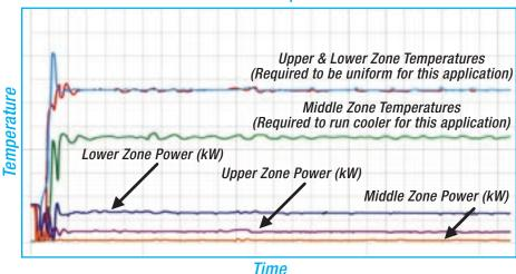
For example, in this particular application, a three zone system, upper and lower zone temperatures are required to be uniform while the middle zone temperature needs to run cooler than the end zones.
