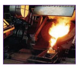
Back slagging as shown in the photo simplifies slagging by eliminating the need to lift heavy slag from the melt or drag it through the pouring spout. The back slagging feature permits the furnace to tilt at a 33° angle towards the rear. Tilting the furnace provides sufficient space above the deck for a portable hopper and makes it easy for the slag to be pulled through the rear spout into the hopper.
