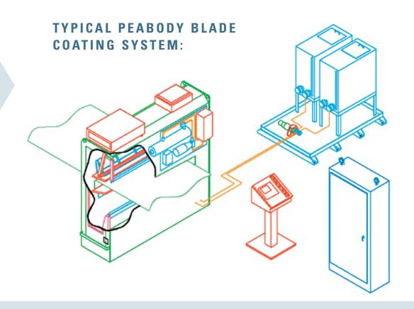
**HERE'S HOW THEY WORK:** In our Electrostatic Systems, coating particles are subjected to a high electrical charge so the now like-charged particles break up into tiny droplets. The charged particles are then strongly attracted to the surface being coated, allowing for controlled, uniform dispersion. What you get is an extremely efficient coating with minimum waste, resulting in substantial cost savings.
