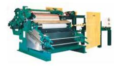
**S-TYPE FINISH COATER:** Finish Coaters can be used individually or in conjunction with each other on separate floors to increase the flexibility and speed of color changes. The configuration can include a S-Type Finish Coater and a T-Type Finish Coater. Addition of the computerized coating head control system allows for roll position and force to be automatically adjusted and controlled.
