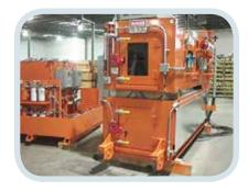
**ROTARY ATOMIZER SYSTEMS:** In Rotary Atomizer Systems coating is delivered to a rotating bowl, then spun out to the bowl's edge where it is subjected to an intense electrostatic energy field. The patented atomizer is rotated at high speeds using a friction-free air turbine. A combination of centrifugal and electrostatic energy is used to atomize and distribute coating fluids uniformly over the target surface.
