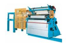
**PRIME COATER:** This conventional "S" Type Prime Coater includes a retractable topside head. Teamed with the GFG cantilever applicator roll removal feature, the Prime Coater allows for easy replacement of the bottom-side applicator roll.
