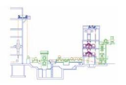
**BLANK PROCESSING LINE**: GFG has teamed up with robotic integrators to produce the highest quality Blank Processing System capable of automatically loading automotive blanks on to a conveyance system that transports the blanks through a GFG wash, rinse and drying section. Once cleaned, the blank then progresses through a GFG - Peabody Electrostatic Oiler that applies a specific amount of stamping oil to both sides of the blank before being off-loaded by the robotic unload station.
