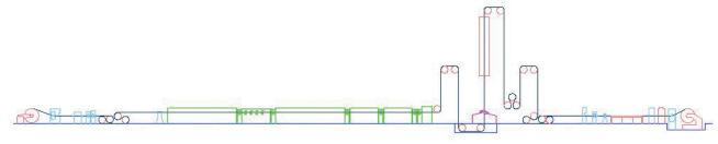
**PAINT COATING LINES:** GFG has designed, built and installed Paint Coating Lines in various configurations. One of the most versatile line configurations is shown below complete with a Chemical Coater, Prime Coater, Finish "A" and Finish "B" Coater. By utilizing the combination of Finish "A" and Finish "B" Coater color changes can be made "on the fly" with virtually no scrap and no down time. Other GFG line configurations include vertical coaters and wet sections, and Z Line configurations.
