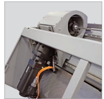
▲ Mandrel bending unit freely programmable over entire tube feed length
