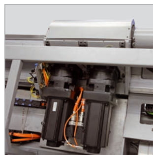
▲ Tube positioning with boost pressure function of advance feed unit
