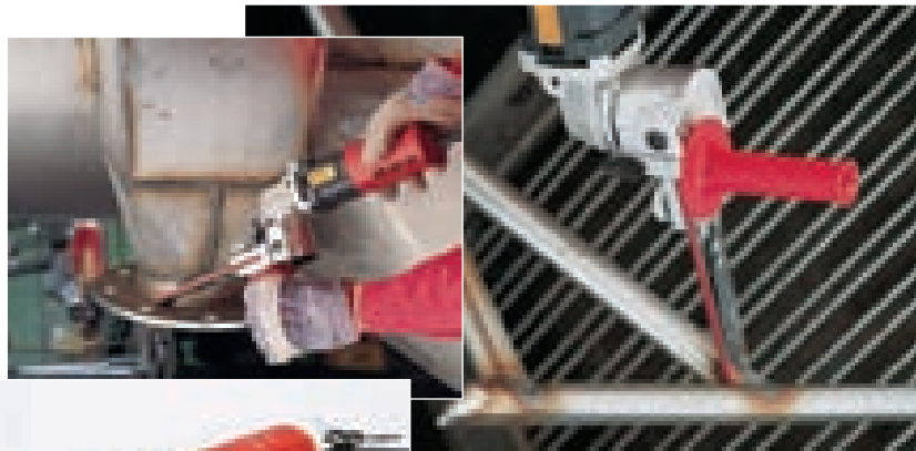
Narrow filing arm and 140° adjustability allow sanding and grinding in confined and difficult areas.
