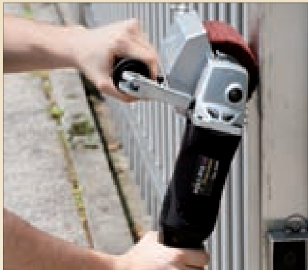
Satin finishing using interleaf fleece wheel.
