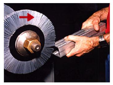
Deburring with a radial wheel brush can be either an off-hand process or machine based. Limitations of offhand deburring include low productivity, irregular quality and potential for operator injury. Due to these factors, off-hand deburring of PM parts is rarely, if ever, employed.
