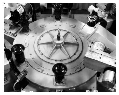
Figure 6: Rotary table deburring system
