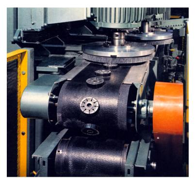
Figure 9: Close-up of disc brush deburring system
