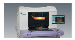
This addition to our automatic optical inspection department enhances our ability to scan both inner and outer layers to the highest degree of accuracy.
