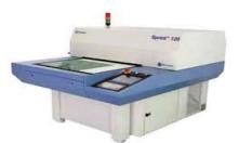
With this addition PCB and panel traceability is assured with multiple serialization and bar-coding options defined per panel, strip or individual PCB. Located in the clean room of our screening department the Inkjet offers piece to piece consistency of image print & accuracy.
