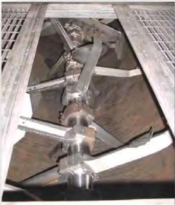
**Rugged Cast Arms that are Mechanically Fastened to the Agitator Shaft**
