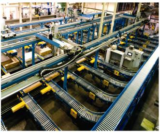
Centralized Gantry Robot Palletizing: Ideal for many simultaneous products at low rates. Compact footprint and telescoping z-axis for low ceiling areas, with high speed sortation.
