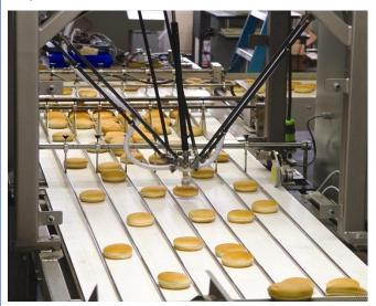
High Speed Packaging: Vision guided picking and placing up to 50 products per minute.
