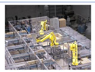
Centralized Pedestal Robot Palletizing: Flexible packaging of multiple lanes at moderate rates.
