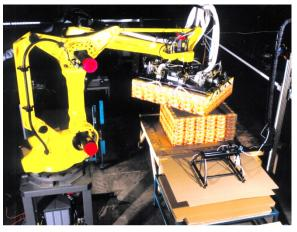
Robotic Unitizing System: High speed layer palletizing. Includes slip sheet, tier sheet, and/or cap handling options.
