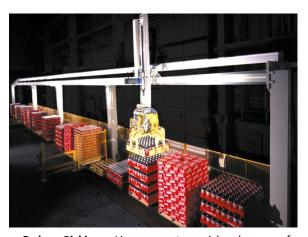
Order Picking: Linear gantry picks layers of containerized product to build mixed pallets that are placed on delivery trucks.
