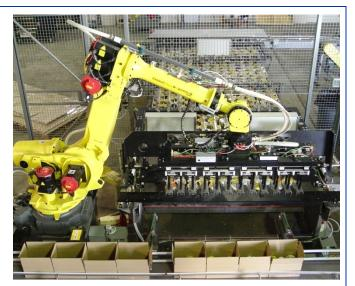
**Robotic Case Packing:** For products that are difficult to handle and require unique case packing and cartoning equipment.
