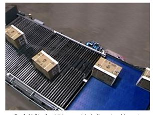
Pack-N-Stack: Vision guided line tracking, tray loading, and stacking within the same system utilizing robot flexibility.
