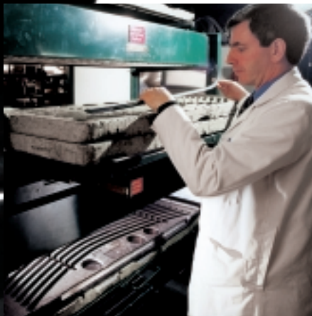
Heating of chrome strips
