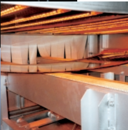
Heating of glass prior to PU-foam application
