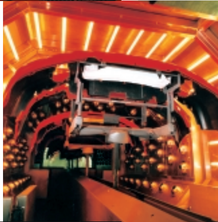
Curing of paint on plastic bumpers
