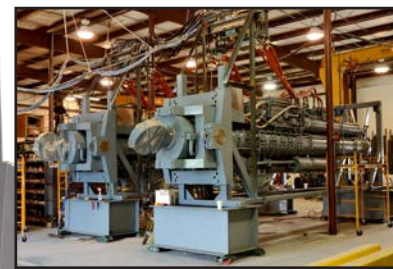
Each of the 51,000 lb. cylinder assemblies required a custom stand for assembly and transportation.
