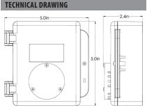
Note: Drawings above are shown with an optional splash guard. Without splash guard, thickness of unit is 2.1" (53.34 mm).
