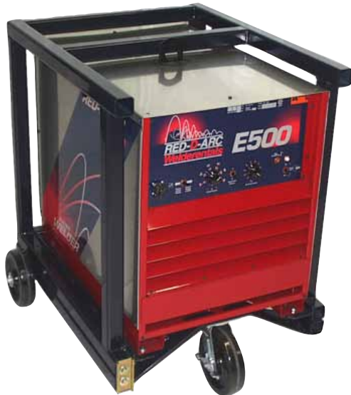
230/460/575 Volt, 60 Hz, 3 Phase Input
