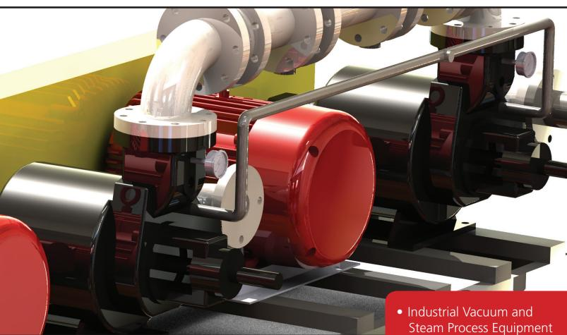
\*Vacuum priming system designed and built by NES Company Inc. for the Picayune Strand Everglades restoration project.
