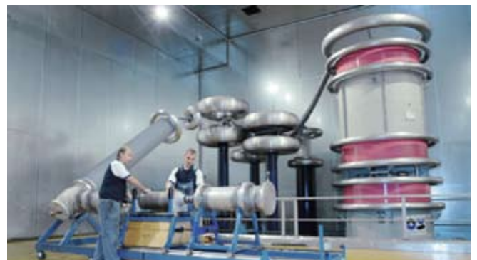
Preparation for a routine test of a SiR slip-on body at our fully screened routine test room
