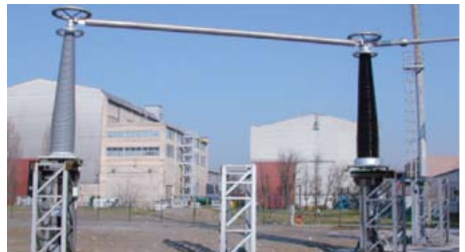
Prequalification test of 420 kV-equipment at the CESI laboratory in Milan, Italy
