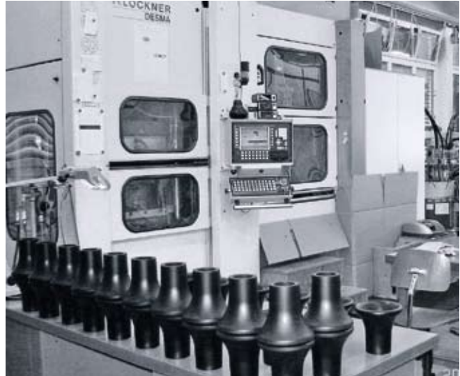
Fully automatic production facility for silicon parts
