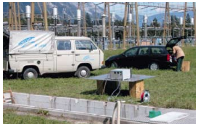
PD measurement on customer in Switzerland
