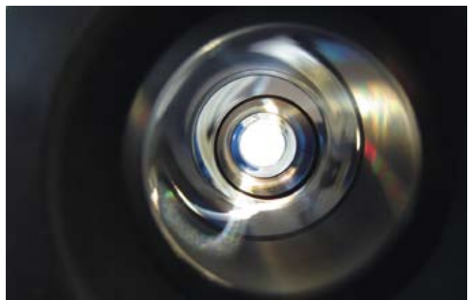
Clean surface in the SiR slip-on joint body
