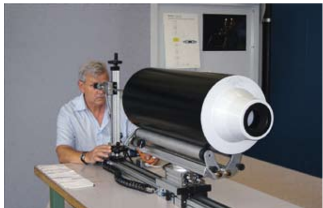
Single control of the surface of a SiR slip-on joint body after production
