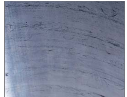
PolySlide cylinder wall surface showed minimal wear.
