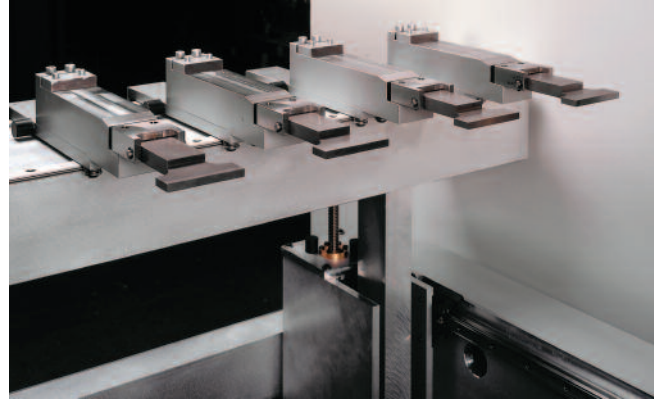
Two-axis backgauge (X-R) with pneumatic clamping for finger placement on PPEB-5
