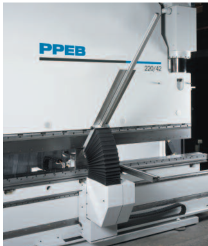
PP8402 T1, T2 CNC sheet supports with CNC vertical adjustment / Standard duty
