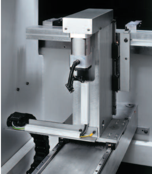
Four-axis backgauge on PPEB-EQ (X-R-Z1-Z2)
