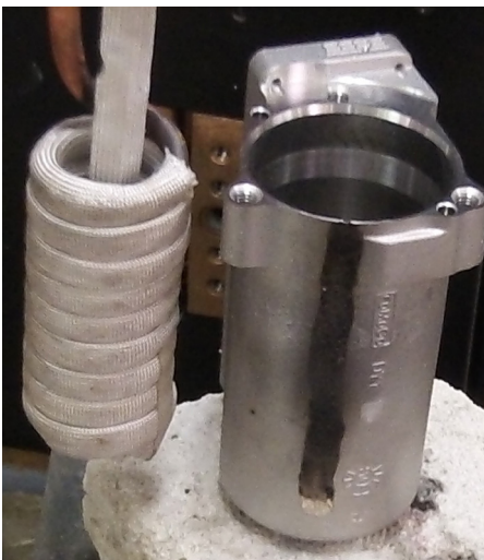
The internal bore coil and the motor housing.
