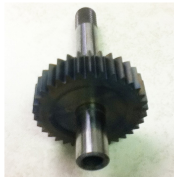
The gear and shaft after shrink fitting.
