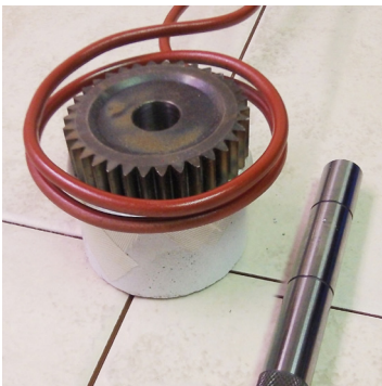
The gear and the shaft prior to heating.
