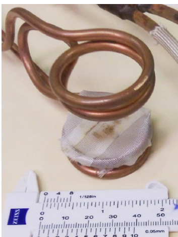
The split helical coil enabled easy loading.
