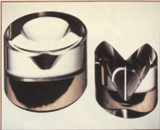
The cone V-bearing allows the pivot some radial freedom while keeping it centered. The bearing may be used vertically or horizontally. The V-block involves greater friction but carries higher load. It is used in scales and balancing mechanism with a knife edge riding in the V.
