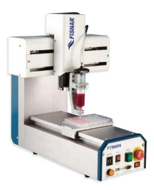
A powerful compact-sized desktop robot with a working area of 7.87" x 7.87" (200 x 200mm). Its reduced benchtop footprint makes it an ideal robot for automating a current manual dispensing application.
