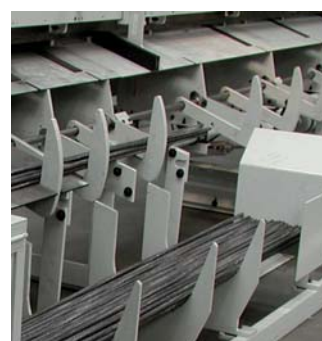
▲ Stop of tilting station and rod-end alignment
