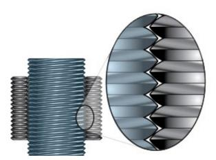
Heat Management – Roller screws have more points of contact which results in more heat because of the increased friction. The benefit is that roller screws have a higher force capability and longer life when compared to ball screws. Roller screws are ideal for repeated stress applications in the same area of actuator stroke, such as pressing, inserting, and riveting.
