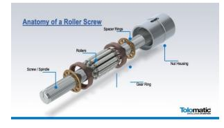
planets. Gear rings and spacers hold the rollers inside the nut. While the rollers are orbiting the screw, a small amount of sliding occurs, which is one of the stark differences from a ball screw. By constraining either the screw or the nut from rotating, this allows the other rotating element to move across the stationary element; thus, creating linear motion in the same way that motion from a ball or acme screw is produced.
