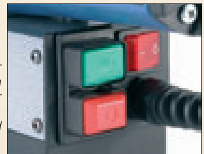
Switches for power and magnet adhesion are arranged for simple, uncomplicated operation.
