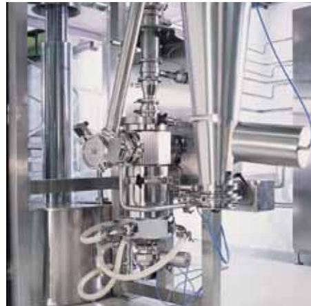
CIP-DESIGN 200/1 AFG SYSTEM FOR MANUFACTURING INHALER LACTOSE WITH CONTROL UNIT AS DEFINED IN 21 CFR PART 11
