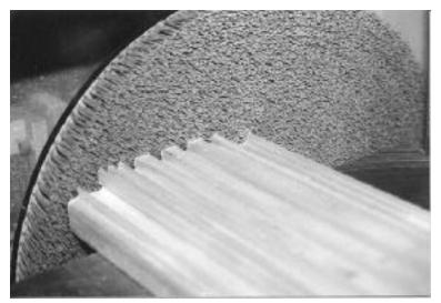
Figure 4 Extrusion Presented to Disc for End Deburring
