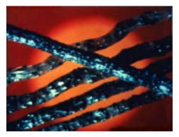
As the filament is applied to the work piece and begins to wear, new abrasive grit is exposed. The filament is, in effect, self sharpening.
