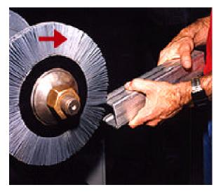
As this entire process is dependent on operator skill, inconsistent finishing is often the result. Variables such as depth of penetration, dwell time, and angle of attack are all uncontrolled. Furthermore, because this is
