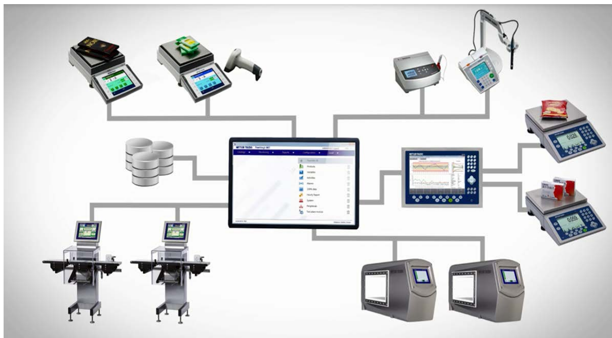
Figure 6: Statistical quality control software such as FreeWeigh.Net integrates data capture and analysis for many devices including checkweighers and analytical instruments.
