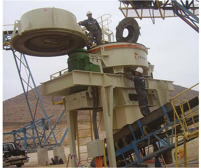
The Barmac B-Series VSI is designed with ease of installation in mind.
