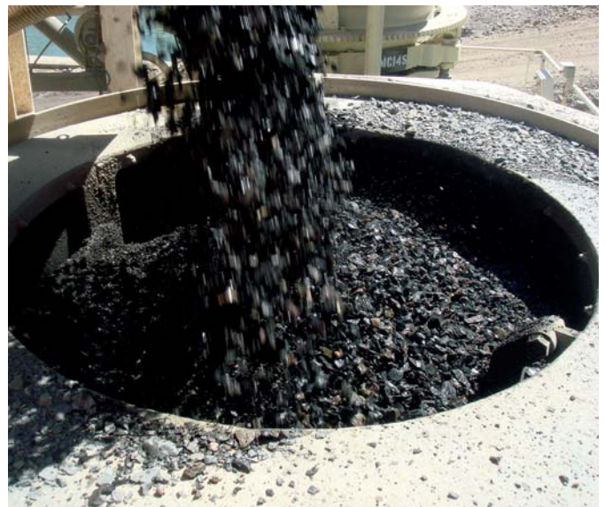
Material may be introduced into the crushing chamber via cascade, thus bypassing the rotor.
