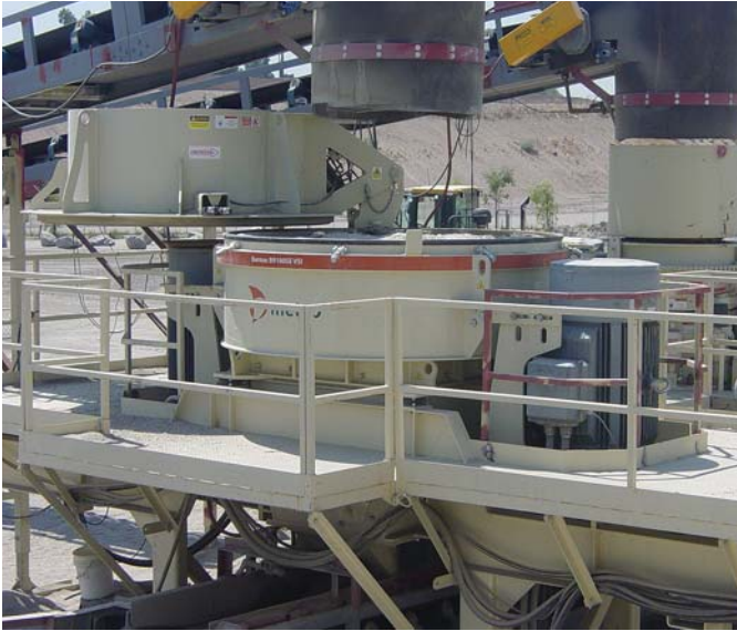
The Barmac B-Series VSI's roof lifter allows easy access for servicing the machine, ensuring minimal downtime.
