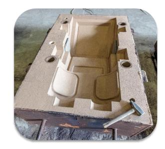
The biggest limitation of sand casting is the need to pull the pattern out of the sand. First, this prohibits features that create re-entrants, unless special cores are added, which increases the cost of the process. Second, there is a risk of dragging sand out with the pattern. To address this, vertical surfaces must have a draft angle added to enable easy release.
