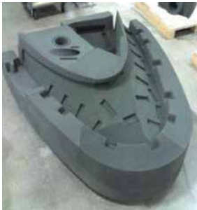
This partially assembled sand-casting mold is being used in the discovery of cost-effective methods to produce phased-out casting designs that are still essential for the DoD.
