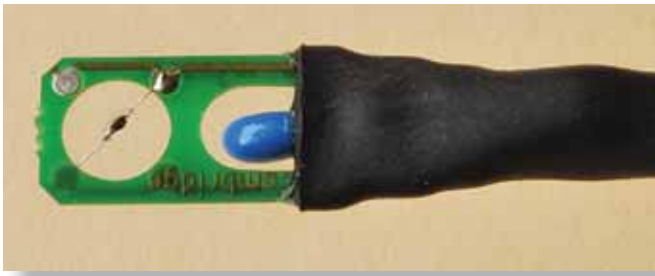
Figure 1. In biosafety cabinets using sensor-based airflow control, a thermal anemometer measures the downflow velocity in a single spot in the work surface.
