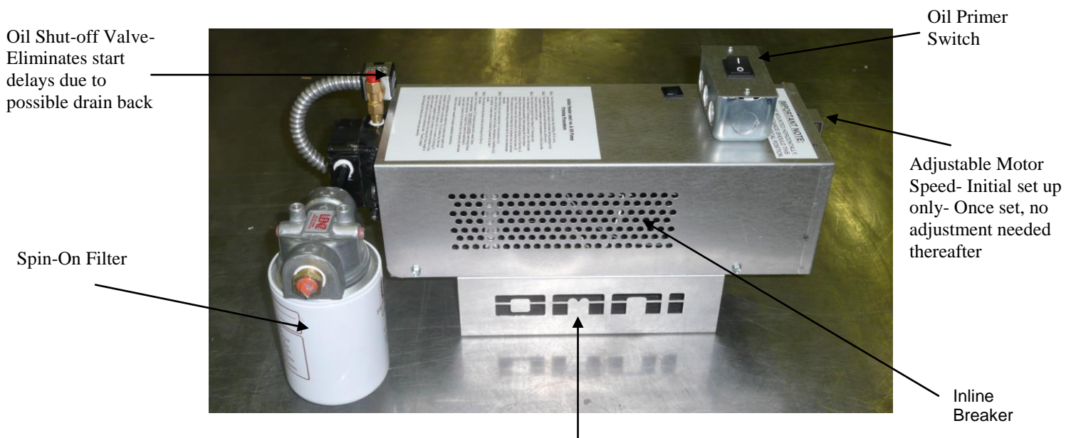
Figure 5 –Oil Pump Assembly
