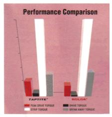
All tests performed with 3/8\*-16 x 1" unslotted hex washer head under controlled laboratory conditions.
