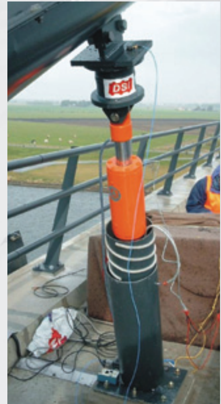
Test Installation of a Hydraulic Damper
