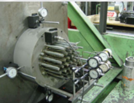
Anchorage of a Fatigue Test
