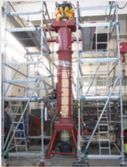
Leak Tightness Test at DSI Laboratory
