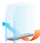
Conventional all-metal spacer allows heat loss through the edge of the glass.
