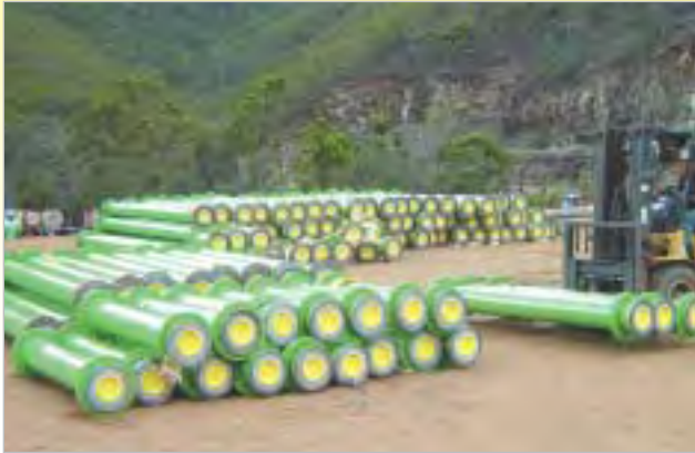
Highly wear resistant ALRESIST pipe used for ore slurry conveying at a nickel mine in the Far East.
