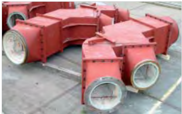
PF-pipes in power plants are subject to significant wear. Despite this fact these areas must not be allowed to fail. In this case the PF-distributors are lined with ALRESIST for high wear and KALCOR for the impact stress.
