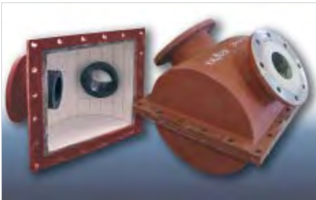
Deviation pot with replaceable ceramic wear protection. This system is used in pneumatic conveying systems where there is little space for large bend radii. It is lined with ALRESIST and ABRESIST.
