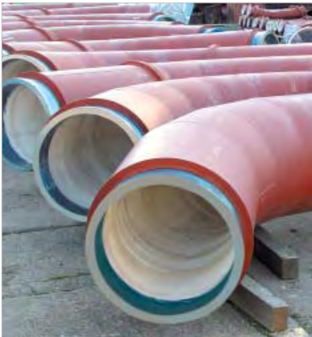
Proven for PF-bends: KALCOR lined elbows and pipe last many years.
