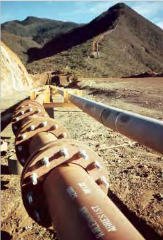
Hydraulic conveying pipeline for ore in Far East.
