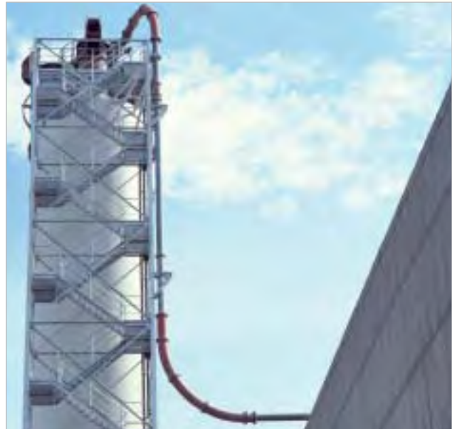
Cement industry example: conveying pipelines to the cement silos are protected by ABRESIST in the bends and subsequent straight sections.
