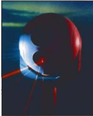
FIGURE 17 Gimbal mounted infrared scanner uses Inductosyn transducers to provide very accurate position information.
