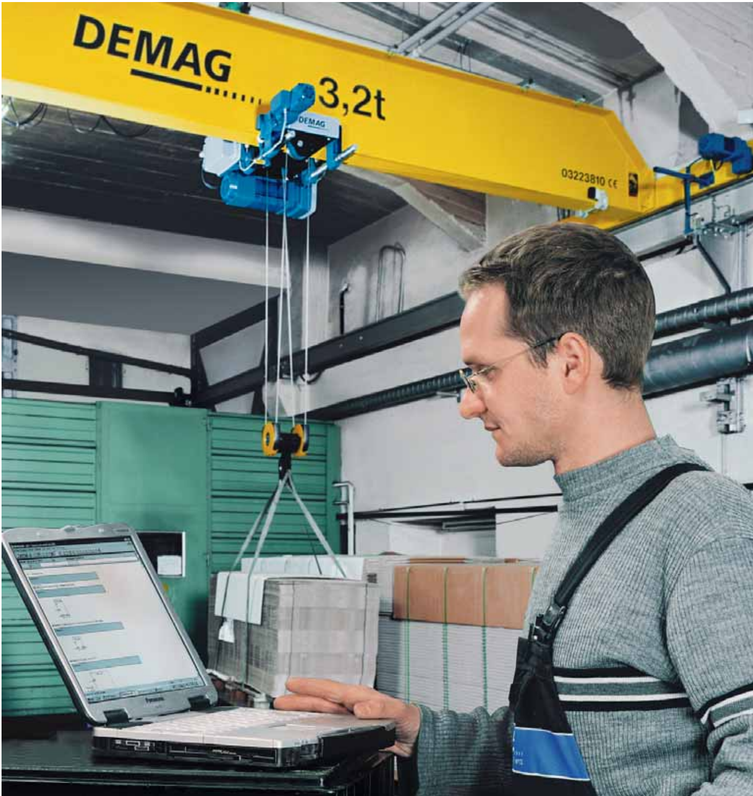
Crane system data can be read out for predictive and scheduled service
