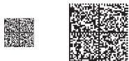
Figure 13: How close does the device need to be to read this 5 mil code and 10 mil code accurately? The key is having the appropriate optical envelope.
