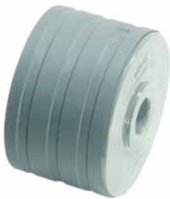
Photo shows a bi-material return roller with 1/2 inch shaft diameter, 1.61 inches length through bore, without flange.
