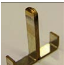
Micro TIG welding bus bars
