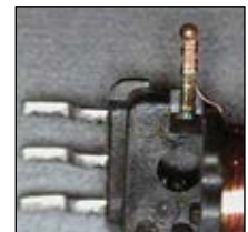
Micro TIG welding motor coil
