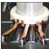
Projection welding radiator connector
