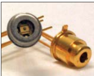
Projection welding small TO devices
