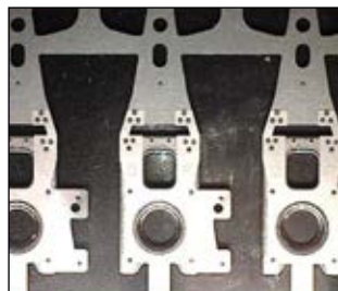
Laser spot welding disk drive arms
