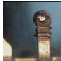
Micro TIG welding magnet wire
