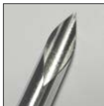
Laser cutting needle
