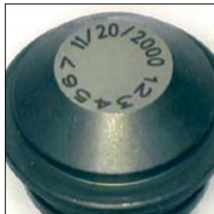
Laser marking on polished steel
