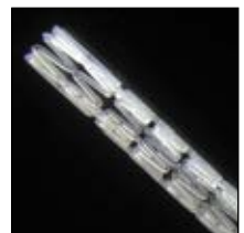
Laser cutting polymer stent
