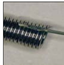
Spot welding wire to coil
