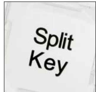
Laser marking on a polycarbonate button
