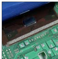
Reflow soldering display FPC to PCB
