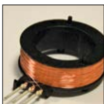
Thermocompression bonding coil wire to terminal
