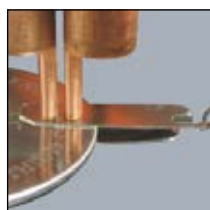
Parallel gap spot welding of coin cell tabs
