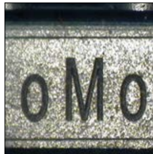
Laser engraving on tool steel
