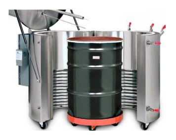
**Step 1:** Place a 55-gallon open top drum onto the drum dolly. Transfer wastewater into the drum to within 6-8 inches of the top. With the evaporator in full open position, roll the drum into the evaporator. Wrap the rope gasket around the drum so that a positive seal will be made when the clamshell walls are closed and secured.
