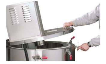
**Step 3:** The evaporator stack is then connected to the flexible section of the permanent exhaust stack with a quick disconnect fitting.
