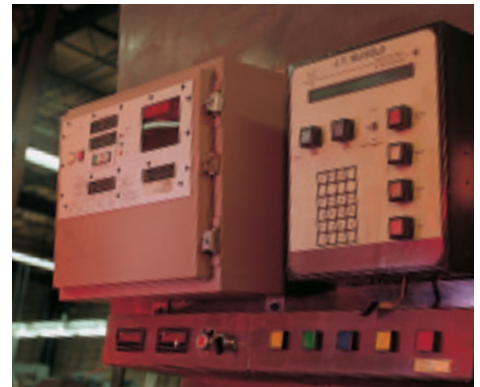
Continuous laser gauging automatically controls rule height.
