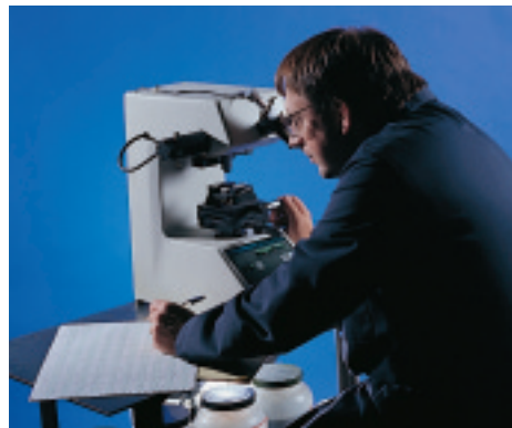
Microhardness testing ensures proper edge hardness.
