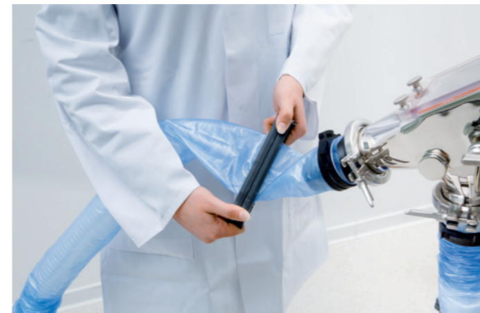
Liner system as the connecting element between the individual system components
