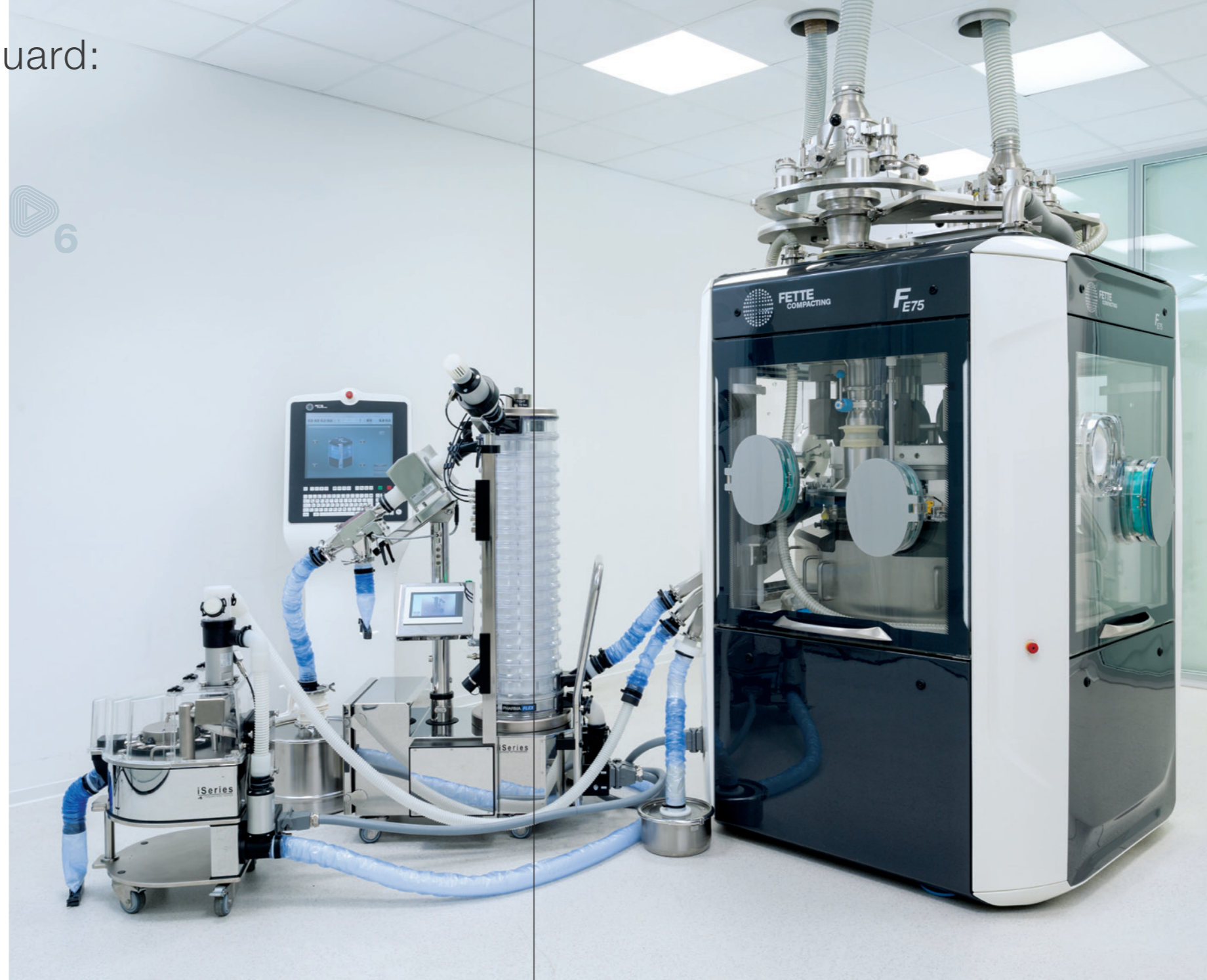
FE75 in 2-layer production with containment package and corresponding process equipment
