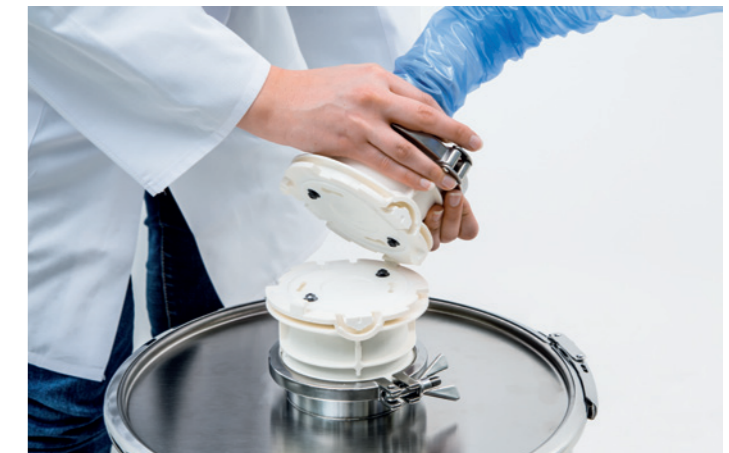
Single-use containment valves for connection to the tablet containers
