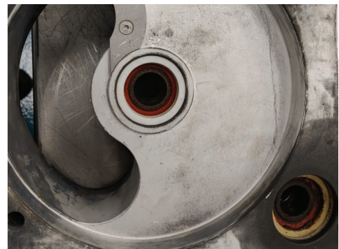
Images of Fill-O-Matic castings damaged by CIP and improper paddle removal tools.
