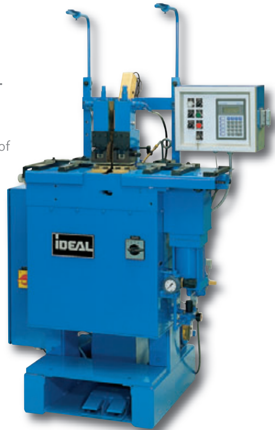
Type BAS 100 with Thyristor annealing device and electronic parameter control
