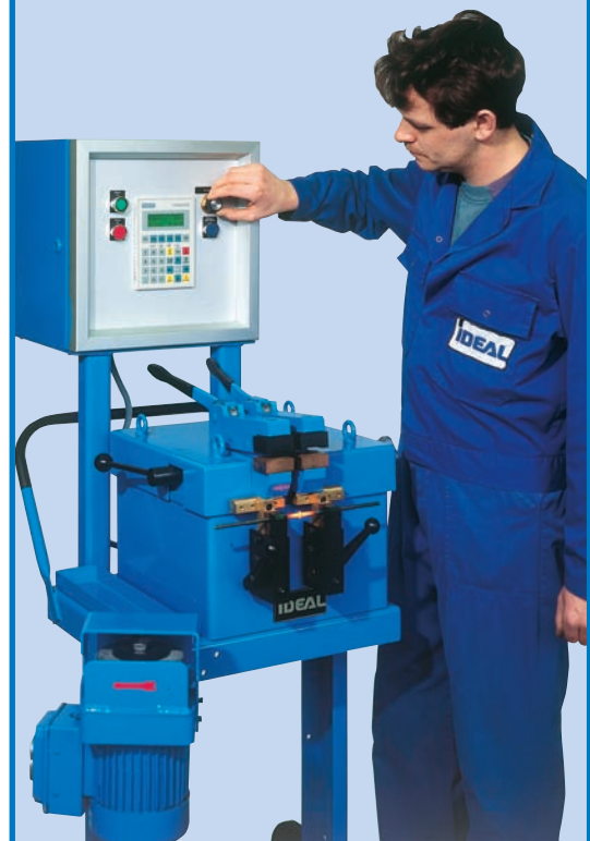
DSH 090 with automatic anneal device GSS, with operator
