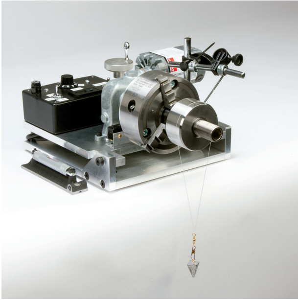
Figure 1a. Typical string method assembly with test shaft mounted.
