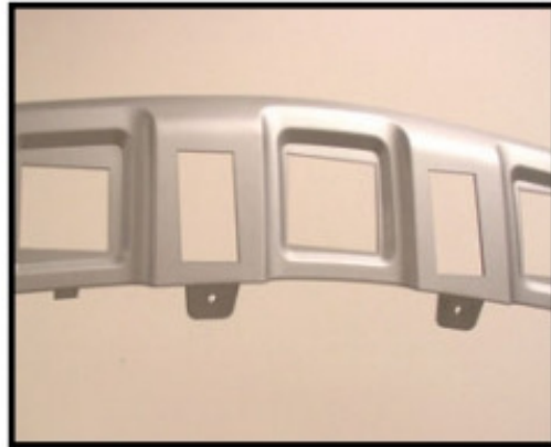
This automotive part exhibits cleanly cut edges after trimming operations using 400 watts of power at a cut velocity of 150 inches per minute.
