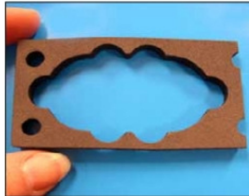
Using a Synrad 100W laser customized gaskets were easily created from a 6.5mm thick sheet of Ethylene-vinyl acetate (EVA) foam.
