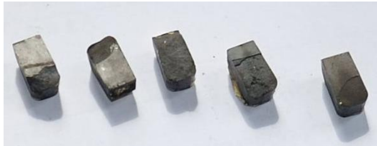
(a) Fracture of PCD Tool Tips in First Test
