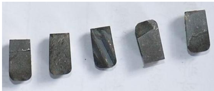
(b) Fracture of PCD Tool Tip in Second Test
