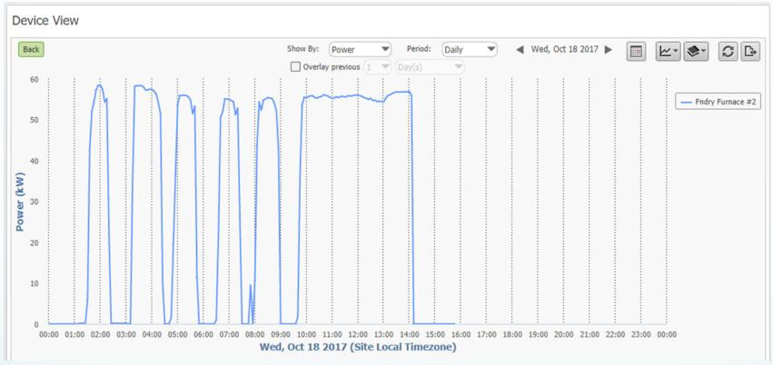
Furnace heating cycle to maintain temperature is typically 1 hour. At 10:00am this furnace remained at maximum load until an alert was sent and the operator shut it down. If this patterned continued over time heating elements would fail. This data provided not only an alert to the operator it allowed management to view energy waste and address plant operations.
