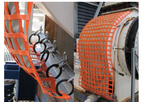
Kevlar safety blankets designed & fabricated by US Netting.
