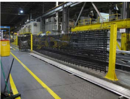
Custom Safety Barrier net for logging facility.
